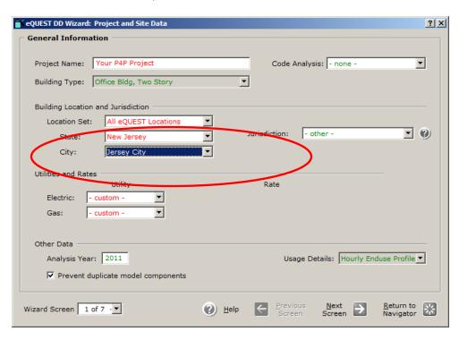
The TMY2 weather station used in the simulation may be found by reviewing the project inputs in eQUEST *Detailed Interface*. To find out which weather file was used, select Project & Site object group, and double-click on Project node in the component tree to open Project Properties window. For example, as seen in the screenshot below, TMY2 file for Newark was used for a project located in Jersey City.
